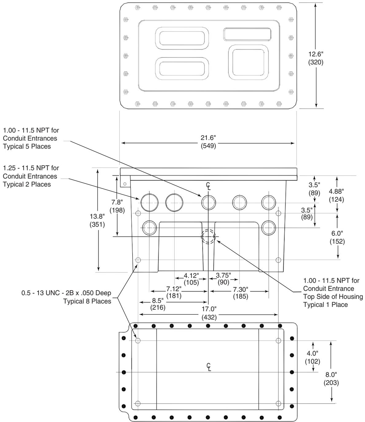
Figure 1 – Explosion-Proof Housing – ALIII-Q Hardware
