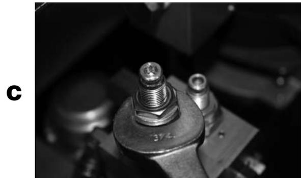
4. Use a  $\frac{3}{16}$ " hex head wrench to turn the adjustment screw in order to reach the correct gauge pressures (D).
