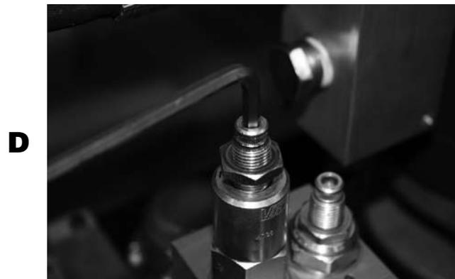
5. Once the pressure has been adjusted, tighten the locking nut and replace the adjustment cover.
