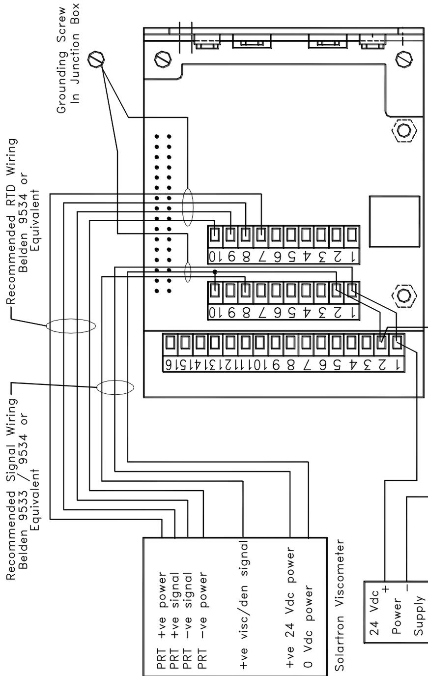
Figure 16. UPCC Solartron Viscometer Head Wiring (Common Power Supply)
