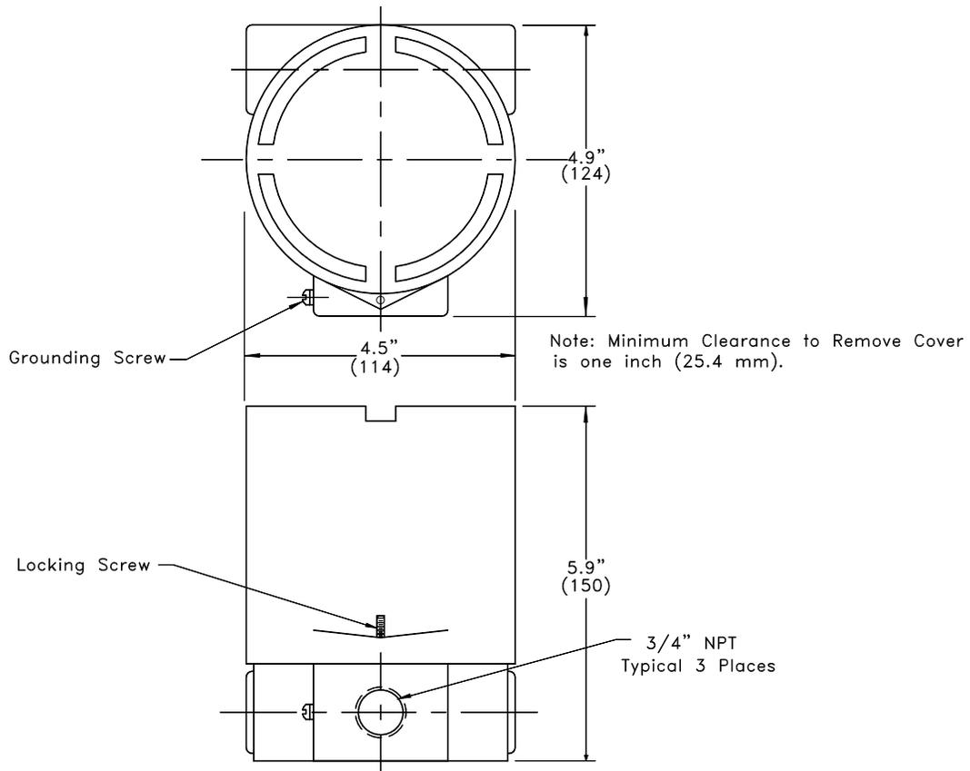
**Figure 2. Explosion Proof Housing Dimensions**
