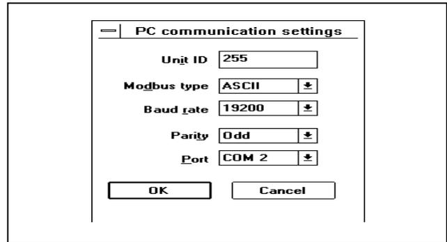
This menu is used to change any PC parameters, such as the Comm Port. For further information, please refer to the “Toolbar Functions (Edit)” section of this manual.
