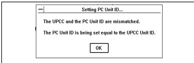
11. Press the “OK” button for the new ID number to be set. The UPCC is now programmed with a unique ID number. Do not try to program another unit with the same number, as this will cause a system malfunction when all units are on the same communications line.
