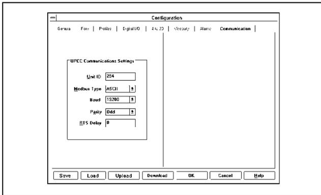
10. To change the Unit ID number, type a new number in the highlighted box, then press “Upload.” Another window will appear, prompting the user to press “Upload.” After the “Upload” button is pressed, the upload procedure will begin. The UPCCMate will then display a warning window as shown below.
