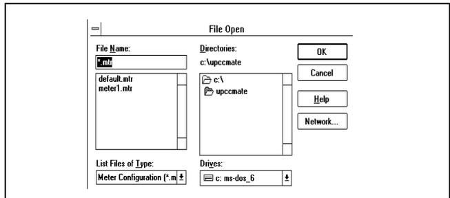
6. This operation will load the default.mtr file parameters into the UPCCMate. The default parameters are used to establish communications with the UPCC on startup.
