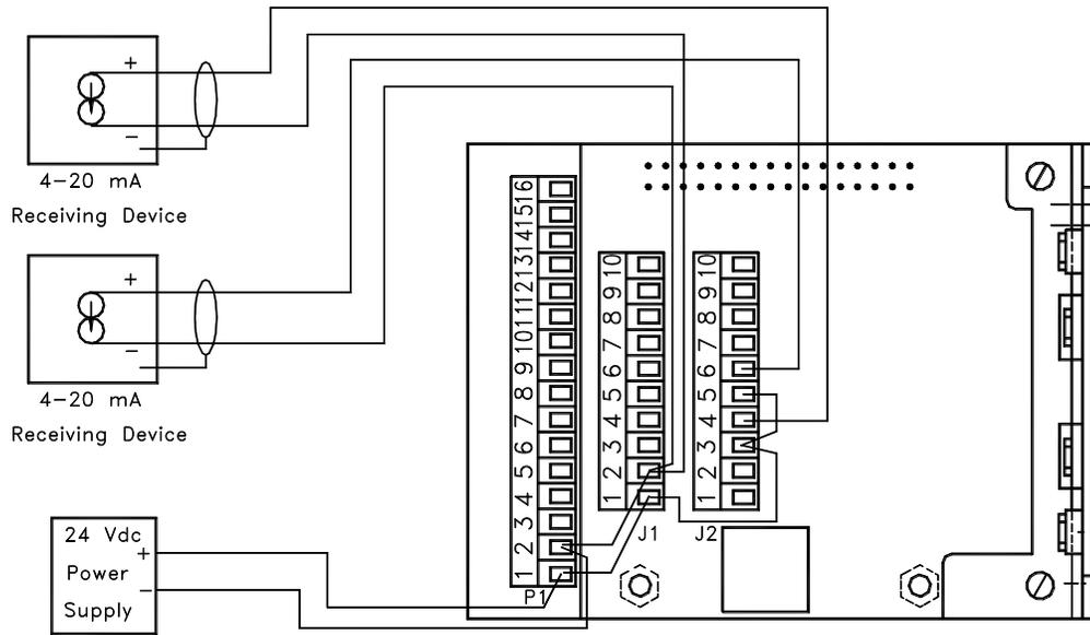
Figure 20. UPCC 4-20 mA Output Wiring
