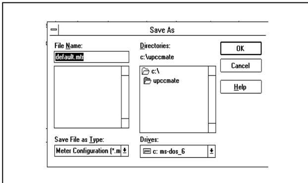
The default.mtr file name is the default name in the “File Name” box. To change the name, press the “delete” key and the box will be blanked. The user can now enter a file name such as meter1. UPCCMate will automatically append the .mtr to the name when the user presses the “Enter” key. For more information on file management, it is recommended that you refer to your Windows documentation as this is beyond the scope of this manual.
