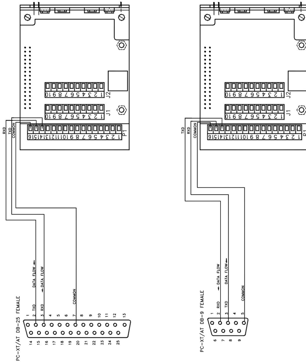
**Figure 11. UPPC EIA-232 Communications Wiring**
