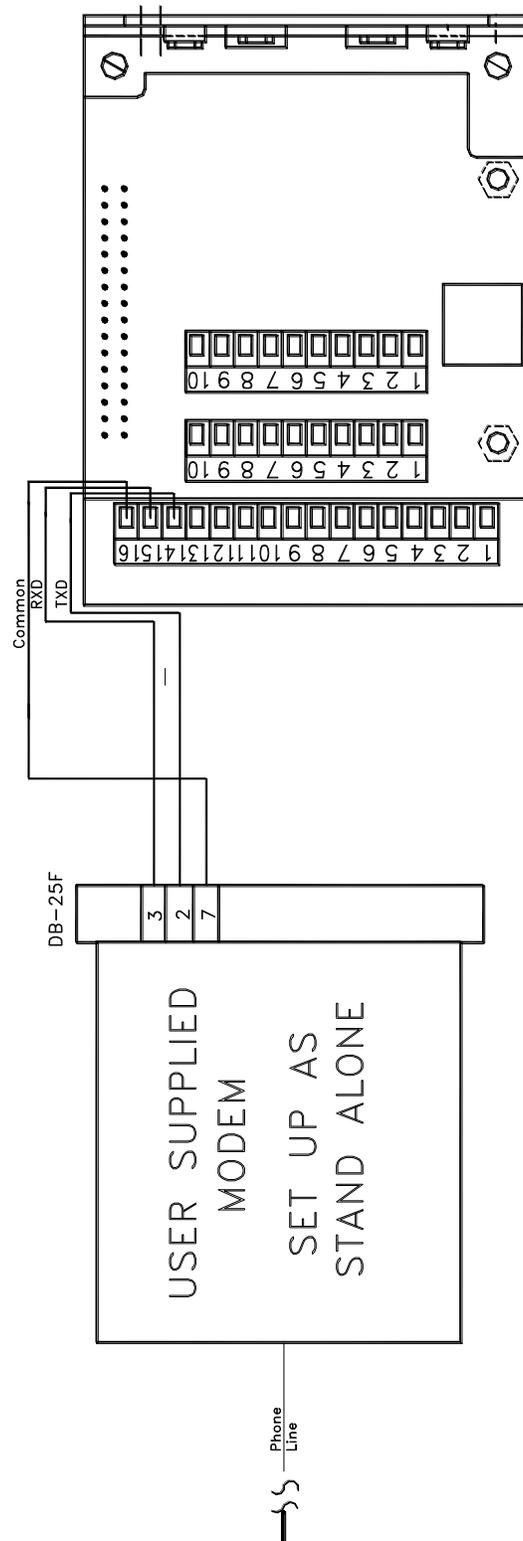
Figure 15. UPCC EIA-232 Communications with Modem
