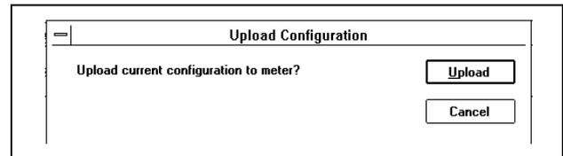
The “Upload” button in this window must be selected to complete the upload. If “Cancel” is pressed, the upload procedure will be aborted and no data will be transferred to the UPCC memory.
