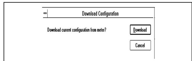
The “Download” button in this window must be pressed to complete the download. If “Cancel” is selected, the download procedure will be aborted, and no data will be transferred from the UPCC memory to the UPCCMate. Once the download procedure is complete, a copy of the data from the UPCC memory is resident in the UPCCMate. The user must save this information to a .mtr file using the “Save” button as described above to save it to the disk.
