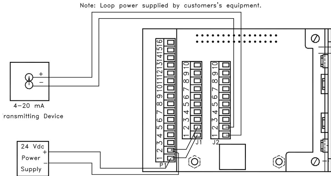
Figure 19. UPCC 4-20 mA Input Wiring
