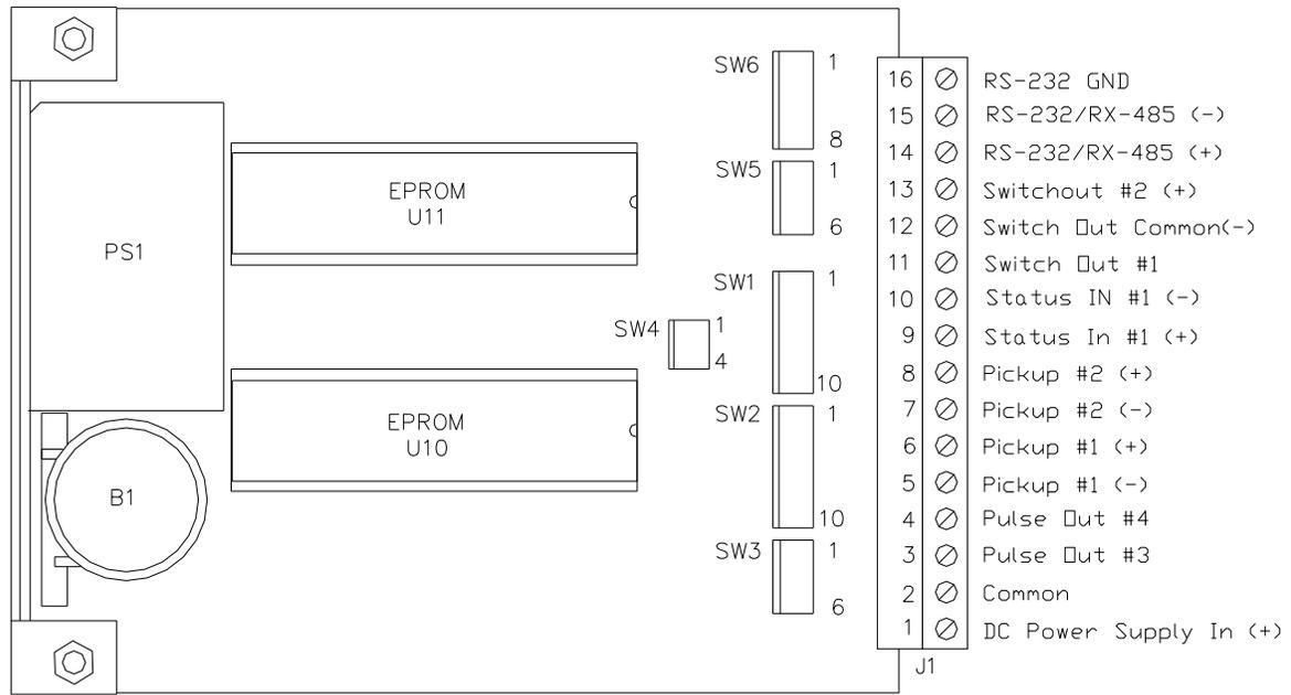
**Figure 6. Switch Locations (Revision 9 and higher Assemblies)**
