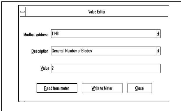
The first is knowing the register number that is to be accessed. (See listing of Modbus Registers in Communications Manual MN02012) The second is scrolling through the descriptions of the registers and then choosing the register based on the description. This screen is segmented into the following windows and buttons:
