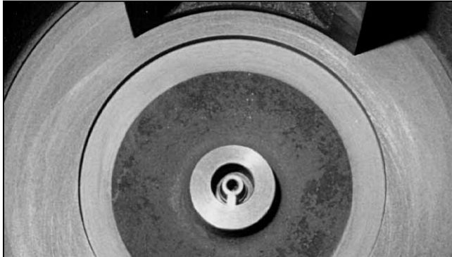
Figure 17 – Cone and Shaft Locking Key in Shaft Socket
