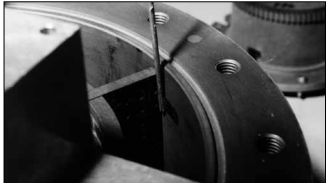
Figure 20 – Measure Blade Tip Clearance
