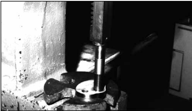
Figure 13 – Press Shaft Out of Cam
