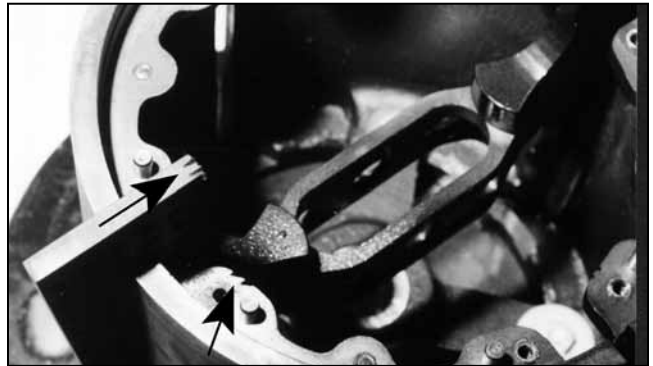
Figure 15 – Locate Blades into their Respective Slots
