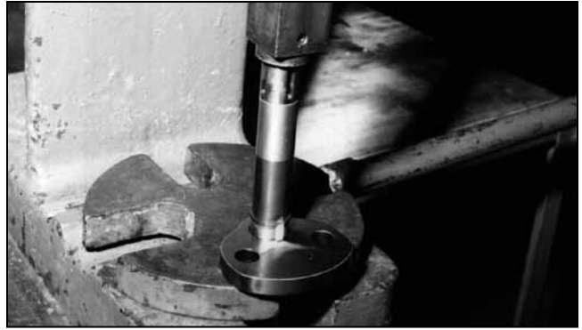
Figure 14 – Press Shaft into Cam
