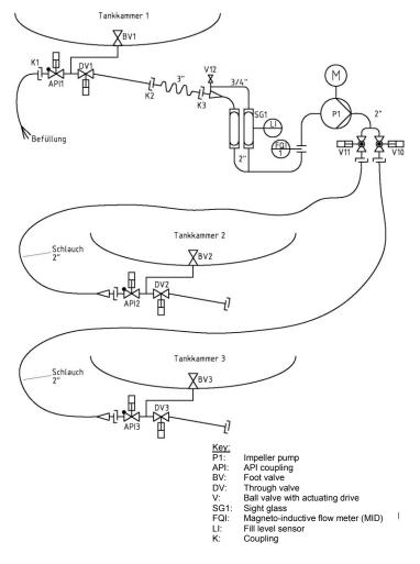
Figure 5: Calibration unit flow chart
