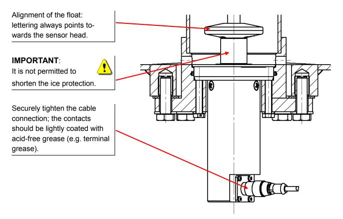
Figure 16: Installation of the sensor head (part 2)
