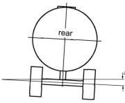
Figure 10: Tank truck negatively inclined in the transverse direction (value: -3.0°).
