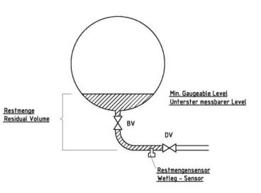
Figure 6: Definition of the residual volume
