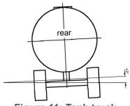
Figure 11: Tank truck positively inclined in the transverse direction (value: +3.0°)
