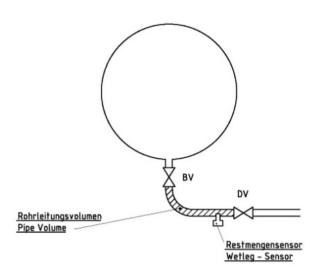
Figure 7: Definition of the pipe volume
