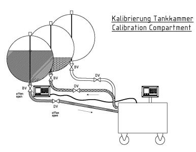
Figure 4: Connection of the calibration unit
