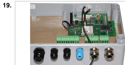
Fig. 2: Standard: only GSM antenna connected
