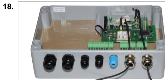
Fig. 1: GSM and Bluetooth antenna connected
