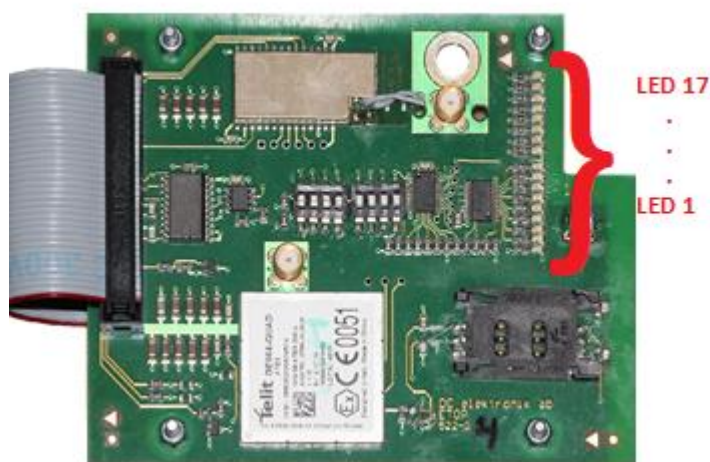
Fig. 6: Communications board with SIM card
